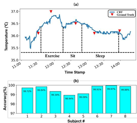
Figure 3: In-Ear thermometer performance evaluation. (a) In-Ear thermometer measured temperature in various conditions; (b) In-Ear thermometer accuracy across subjects.
