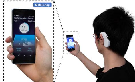
Figure 1: In-Ear Thermometer can monitor the core body temperature by sensing the inside of the auricle.
